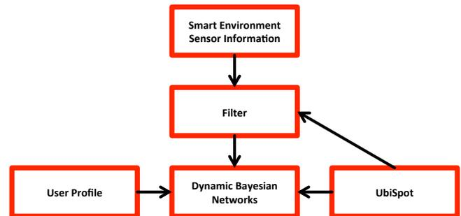
Figure 2. Architecture of the service used for sensor fusion
